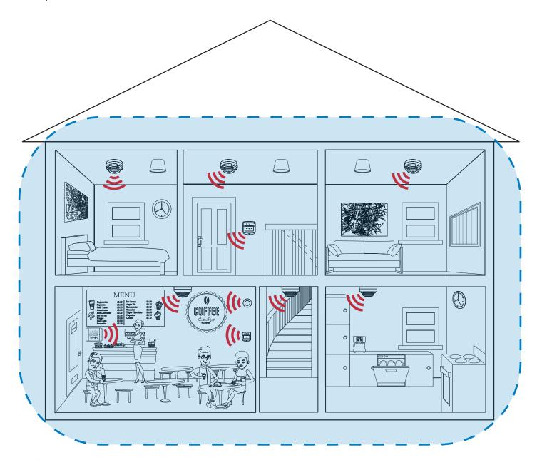
= wireless communication between the SmartCell control panel and the system's fire devices
