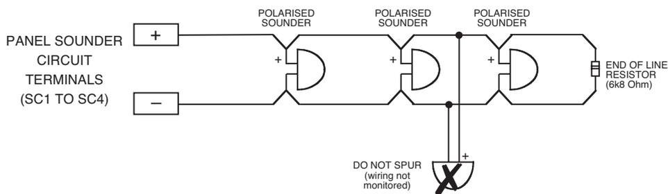
All sounders must be polarised as unpolarised sounders will show a sounder fault. Connect a 6k8 end-of-line (EOL) resistor (provided in the panel’s accessory pack) at the end of each sounder circuit to allow the wiring to be monitored. Unused sounder circuits must also have an EOL resistor fitted at the panel terminals.
