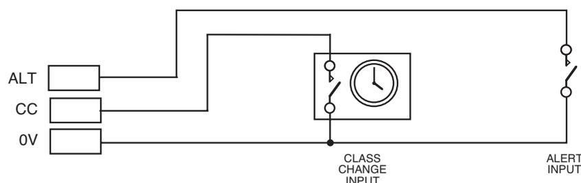
Connect the wiring for each input to the relevant 5mm connector block on the Main Control PCB and terminate their screens at the panel’s base earth distribution post (see page 13 for more details).
