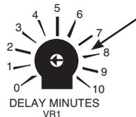
Use a small terminal screwdriver to adjust the delay time period. For information on how to assign individual zones so the delay period applies to them, see pages 16 and 17.
