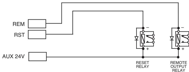
To protect the output stage, only 24V polarised relays with back EMF diodes should be used. If any of the relays are to be used to switch mains potentials, then suitable relays should be chosen and installed and wired accordingly, so as not to compromise the electrical safety of the fire alarm system.
