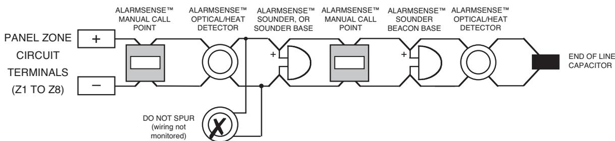
Connect an end-of-line (EOL) capacitor (provided in the panel 's accessory pack) across the terminals of the last device on each circuit to allow the wiring to be monitored. Unused zone circuits must also have an EOL capacitor fitted at the panel terminals.
