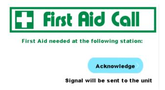
The First Aid screen appears if you press the First Aid button on a call point or the star key on an Auto detector. Press the on screen "Acknowledge" button - this must be pressed and the base station will then send a message back to the unit. The pressed unit will then bleep the sounder and also flash all the LEDS on the call point.
